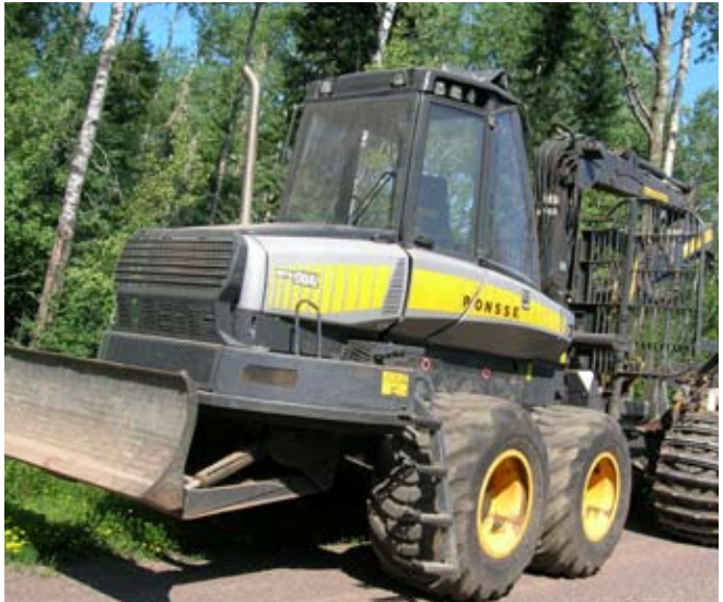
Ponsse Buffalo Dual harvester and forwarder used on many test harvests
