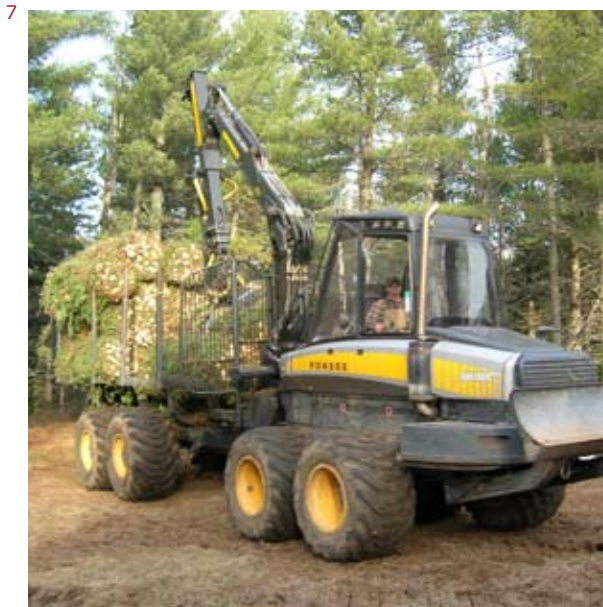
Ponsse Buffalo Dual in forwarding configuration hauling biomass bundles on Pitcha North site
