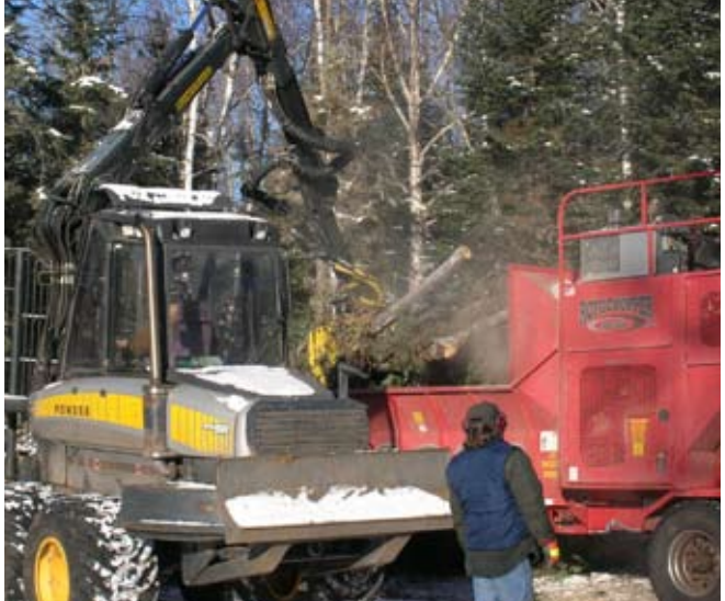
Ponsse Buffalo Dual loading the Rotochopper with loose biomass
