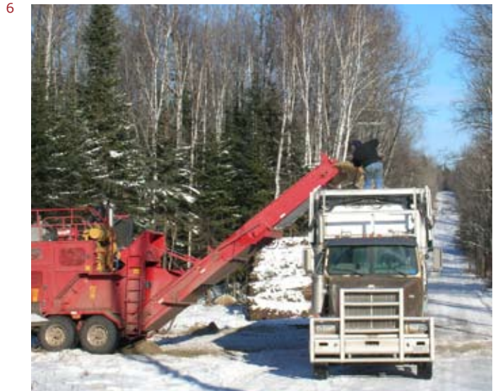
Horizontal Grinder at work on Caribou Trail landing
