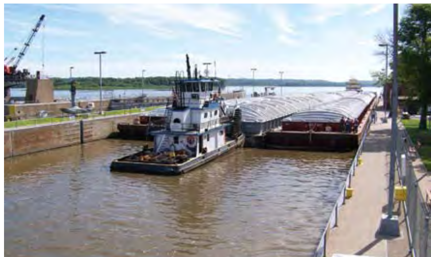
Figure 2: A helper boat prepared to pull the first section of a split tow out of the lock at Dam 16.
