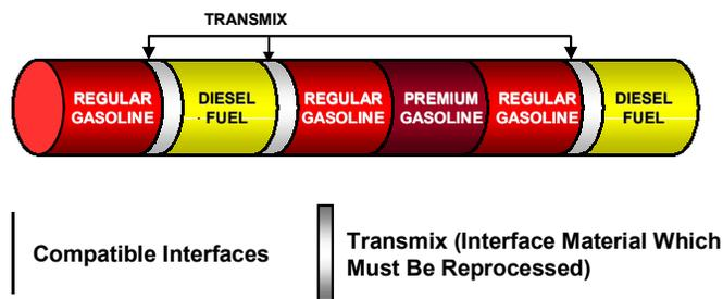
There is always a certain amount of intermixing between the first product and the second at the "interface," the point where they meet. If the products are similar, such as two grades of gasoline, the resulting mixture is added to the lower value product. If the products are dissimilar, such as diesel and gasoline, the "transmix," the hybrid product created by intermixing at the interface, must be channeled to separate storage and reprocessed.
